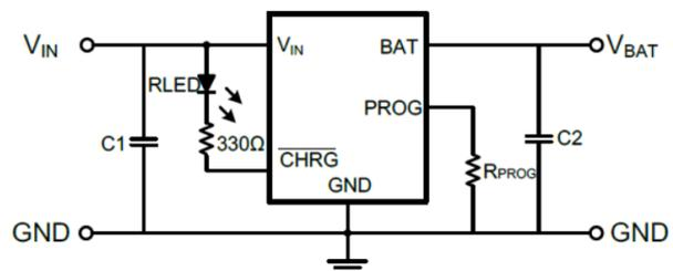
NOTE: C1=4.7µF, C2=10µF,  $I_{BAT}=(V_{PROG}/R_{PROG})*1000$
