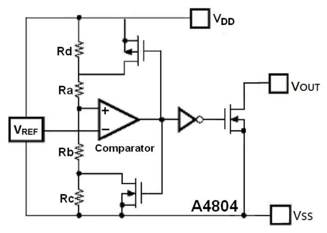
In A4804, a high precision low temperature coefficient reference voltage is applied to the negative input of a comparator. Input voltage, divided by resistor array of Ra, Rb and Rc, is applied to the positive input of the comparator. Output of the comparator controls a pair of NMOS and PMOS switches, generating the hysteresis. Output of the comparator passes a series of buffer to drive the output NMOS.
