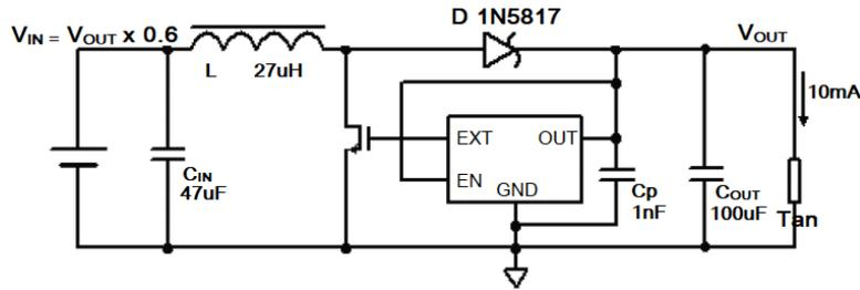
Figure 4. Quiescent current test circuit
