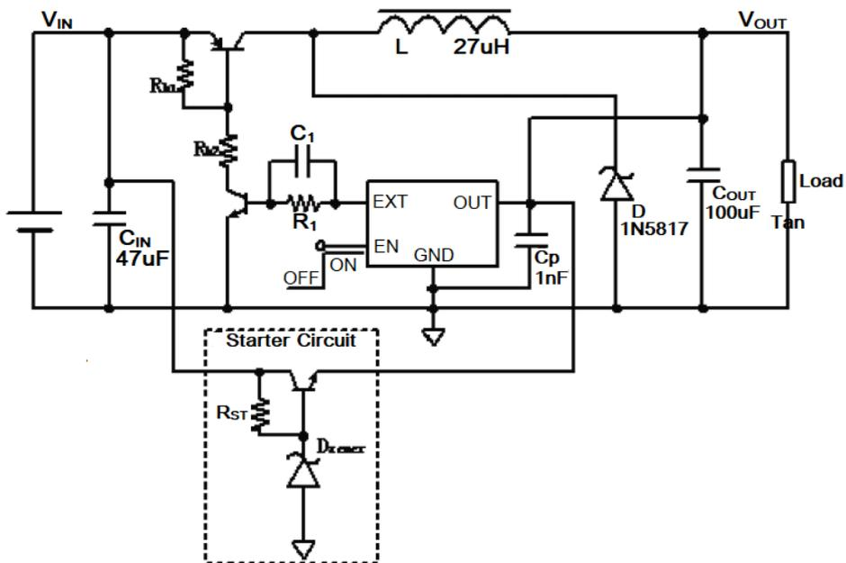
**Note:** In step-down application, use starter circuit as above.  $2.5V \leq V_{zener} \leq V_{OUT}$ . RST is needed for bias current of zener diode. This starter circuit also can be used in high voltage step-up application.
