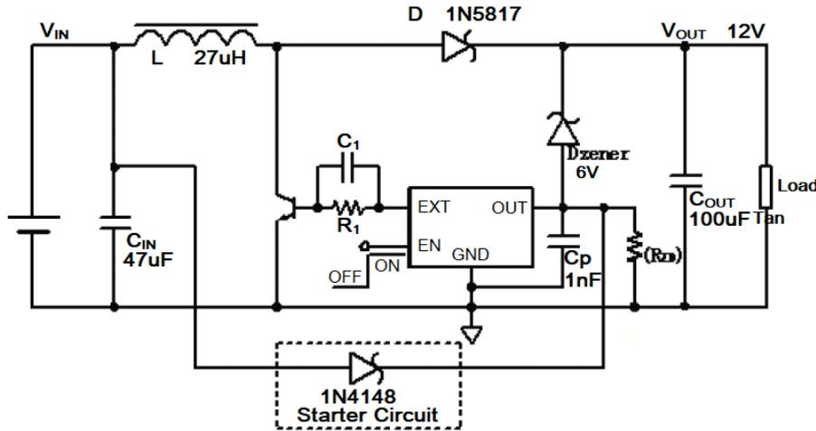
**Note:** A7531's output voltage is 6V. When the output current is small or no load, the output voltage will be unstable, use the RZD for flowing the bias current through the zener diode. For step-up application, a diode (for example: 1N4148) is needed as starter circuit.
