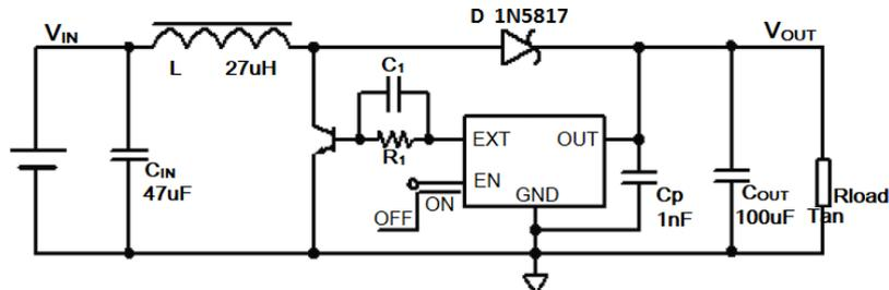
**Note:** R1=330Ω, C1=10nF. (R1 can be calculated by load. If load is light R1's value can be added. If load is heavy R1's value can be smaller.)
