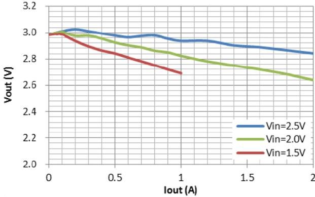
2. Output Voltage vs. Output Current (5.0V)
