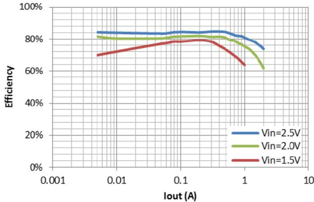
4. Efficiency vs. Output Current (5.0V)
