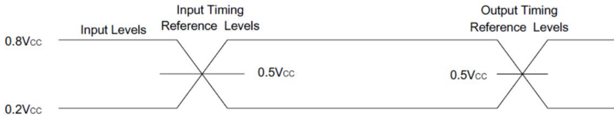
Figure 2. AC Measurement I/O Waveform
