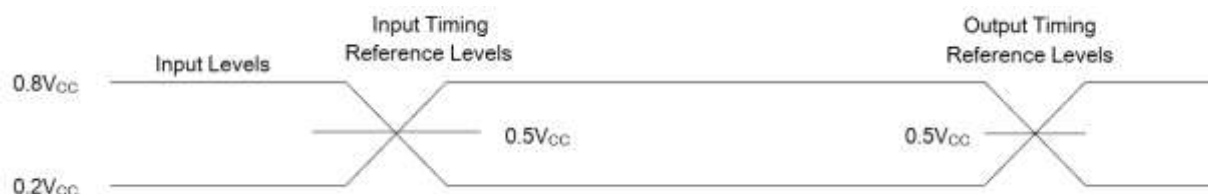
Figure 2. AC Measurement I/O Waveform
