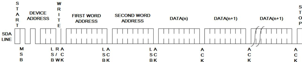
The data word address lower eight bits are internally incremented following the receipt of each data word. The higher data word address bits are not incremented, retaining the memory page row location. When the word address, internally generated, reaches the page boundary, the following byte is placed at the beginning of the same page. If more than 256 data words are transmitted to the EEPROM, the data word address will "roll over" and previous data will be overwritten.
