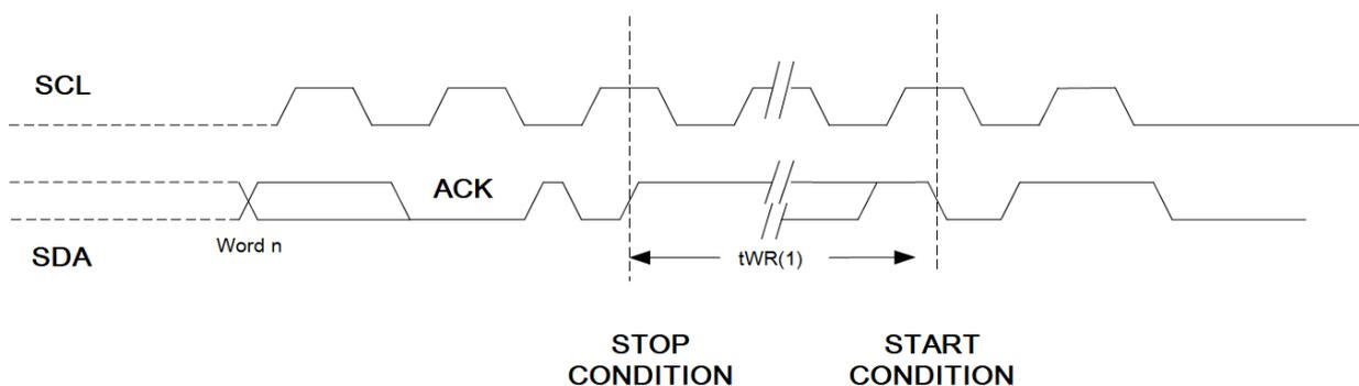
NOTE: The write cycle time  $t_{WR}$  is the time from a valid stop condition of a write sequence to the end of the internal clear/write cycle.
