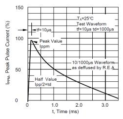
Figure 2. Pulse Derating Curve
