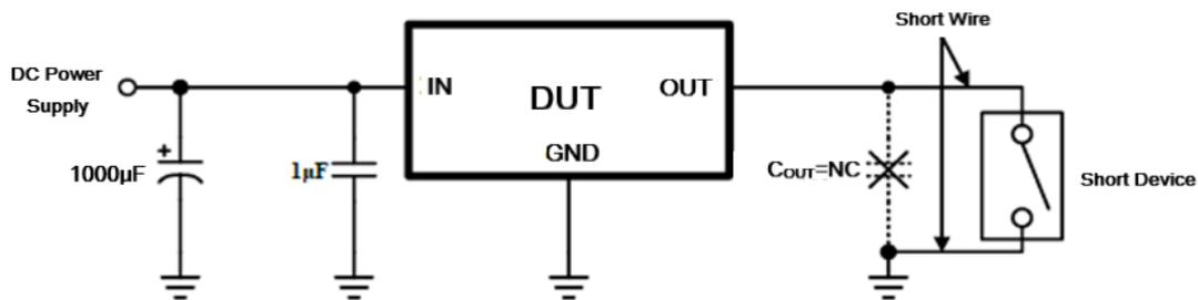
Fig2 Setup to Measure the Short Circuit Characteristic
