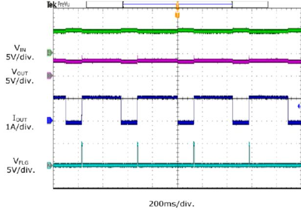
Fig9 Capacitance Load Inrush Response
