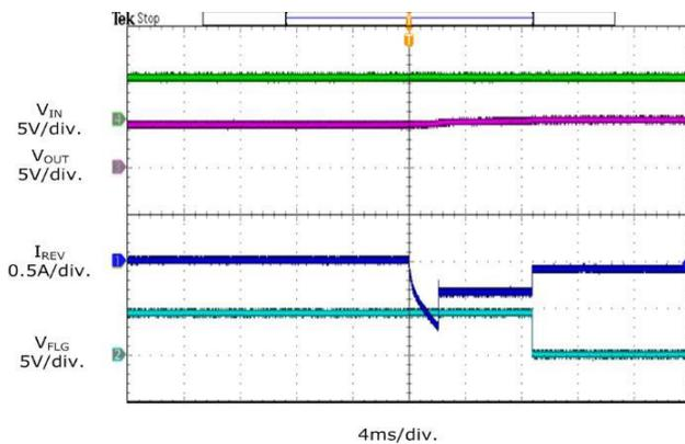
Fig4 Reverse-voltage Protection Recovery
