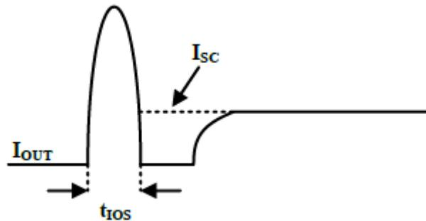
Fig1 Output Current at Short Circuit Moment
