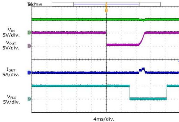
Fig10 Output Current at Short Circuit Moment
