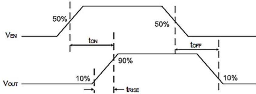
Fig1 Switch Turn-On and Turn-Off Delay Times
