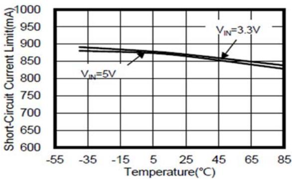
Fig18 Short-Circuit Current Limit vs Input Voltage
