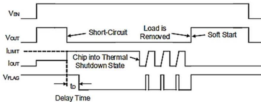
Fig3 Fault Timing: Output Reset by Removing Load
