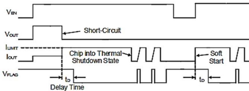
Fig2 Fault Timing: Output Reset by Toggling EN
