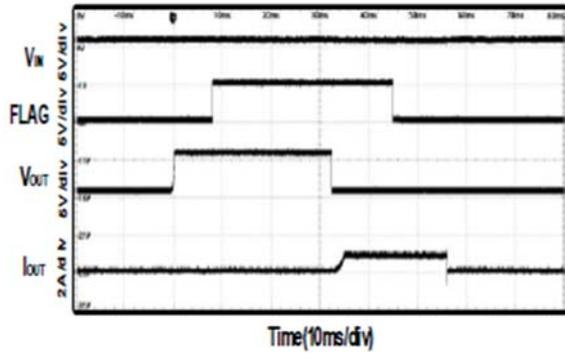
Fig26 Device Enabled into Short-Circuit
