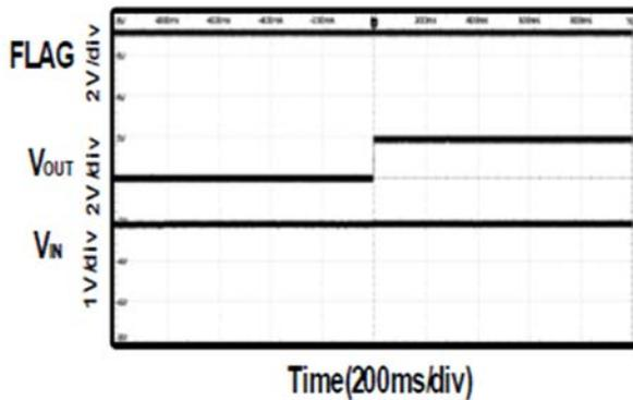
Fig24 UVLO at  $V_{IN}$  Falling
