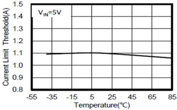
Fig20 Current Limit Threshold vs Temperature
