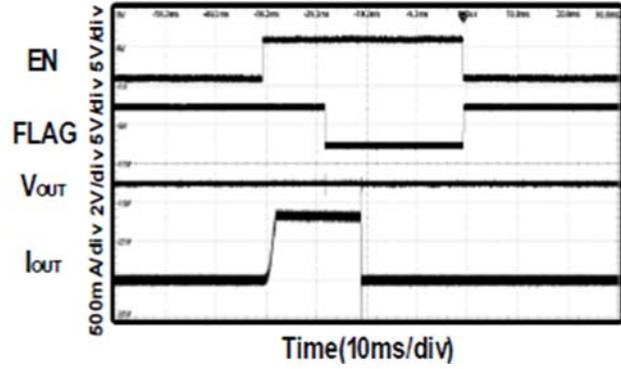
Fig27 Short-Circuit Response Time
