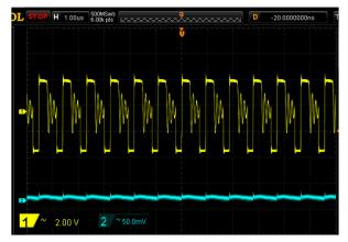
5.  $V_{IN}$ =3V,  $V_{OUT}$ =5V,  $I_{OUT}$ =500mA, CH1= V<sub>SW</sub>, CH2= $\Delta V_{OUT}$
