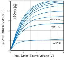
Fig3. Typical Transfer Characteristics
