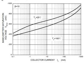
Fig 4.  $V_{\text{CEsat}} \, vs. \, I_{\text{C}}$
