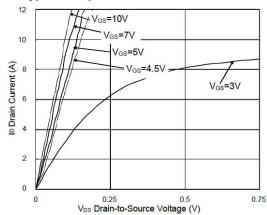
Fig 3. Forward Characteristics of Reverse
