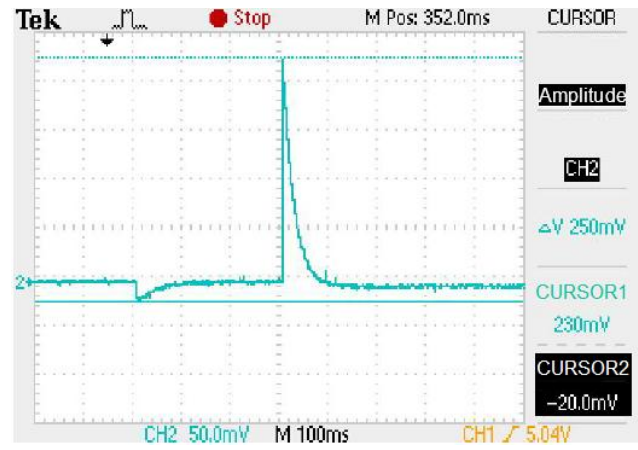
14. Load transient response ( V_{IN}=4.3\text{V} , I_L=0-70-0\text{mA} )
